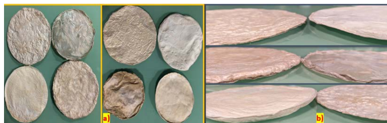
Figure 5. Freeze-dried BCAs without any modification [a] showing the non-homogeneous surface structure of BCAs, b) showing the thicknesses of BCAs].
