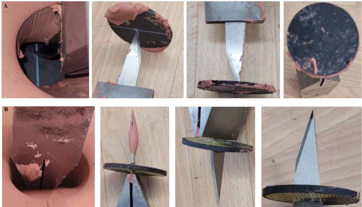
Figure 8: Physical appearance of the 3D printed scales right after impacting drop weight on A) Carbon fiber B) Kevlar fiber from aramid group
