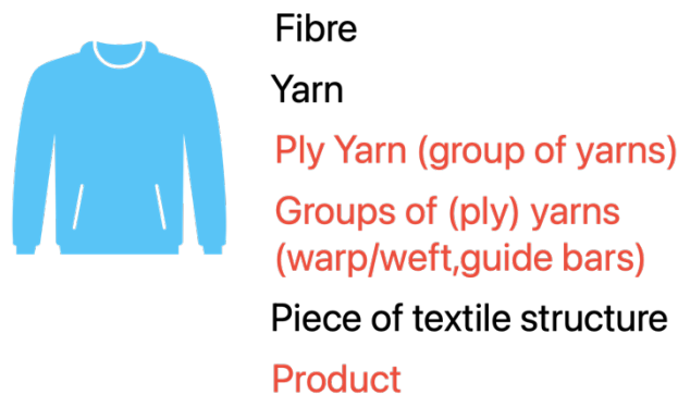
Figure 1. Objects in PyTexLib. The red objects are not implemented for simplicity at the current time
