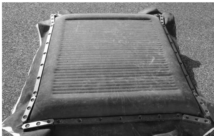
Figure 8. The 3D distance fabric panel during the safety test. In the center there are visible deflections of the skin between binding points that were measured by a laser scanner.
