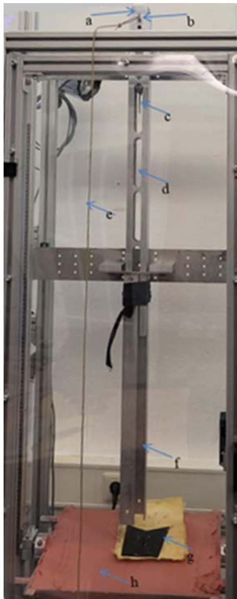
Figure 4: Drop test stand with: a) Dropping weight b) Dropping weight fixing hook c) Knife d) Safety path e) Hook pulling rope f) Safety bar g) Specimen of plastiline h) Plastiline
