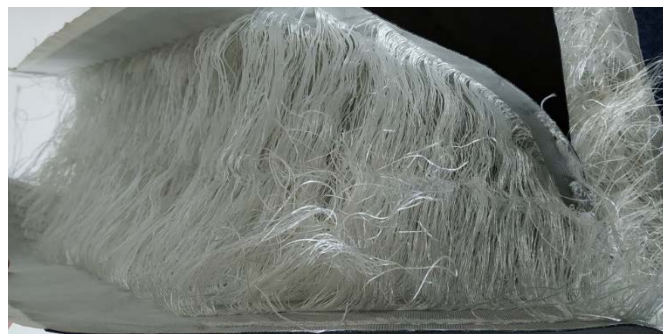
Figure 2. The 3D distance fabric made by Taiwan Textile Research Institute. Total warp pile is 64 650 with different density after warp (150 ends/10 cm) and weft (4.31 ends/ 10 cm). The length of pile yarns is 180 mm.
