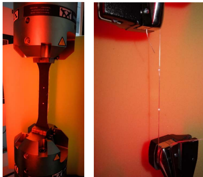
Figure 3: Tensile test of fabric skin and pile yarns using a universal testing machine.
