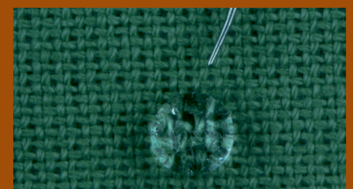
Wetting the surface of a 100% cotton fabric with a pattern created by the combination of hydrophobic and hydrophilic woven and effect threads in the fabric (top: hydrophobic woven pattern + hydrophilic pattern, bottom: both hydrophobic)
