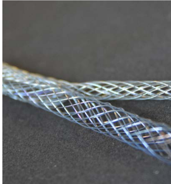
Figure 3. Example for a bifurcated braid
