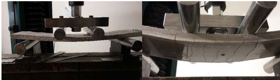
Figure 2. Four-point bending test of geopolymer composite thin plate
