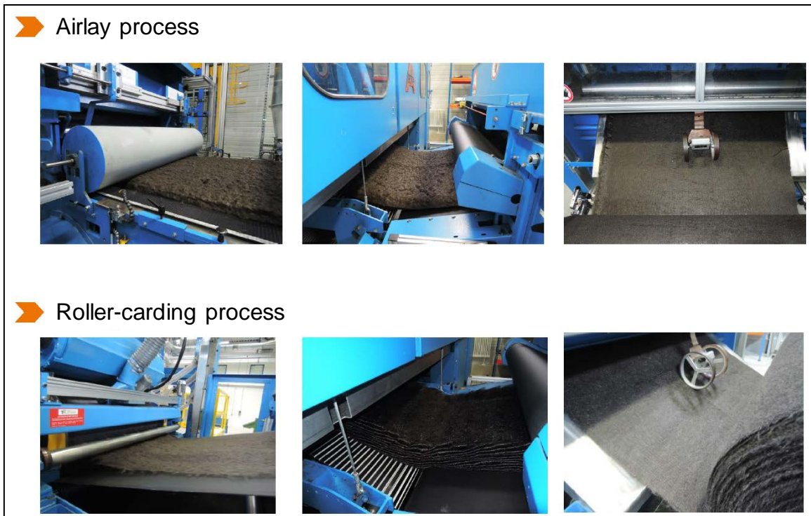
Figure 3. Production of nonwovens from rCF by airlay and roller-carding process.
