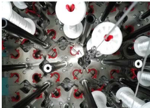
Figure 1. Variation braiding machine with selectable cross sections
