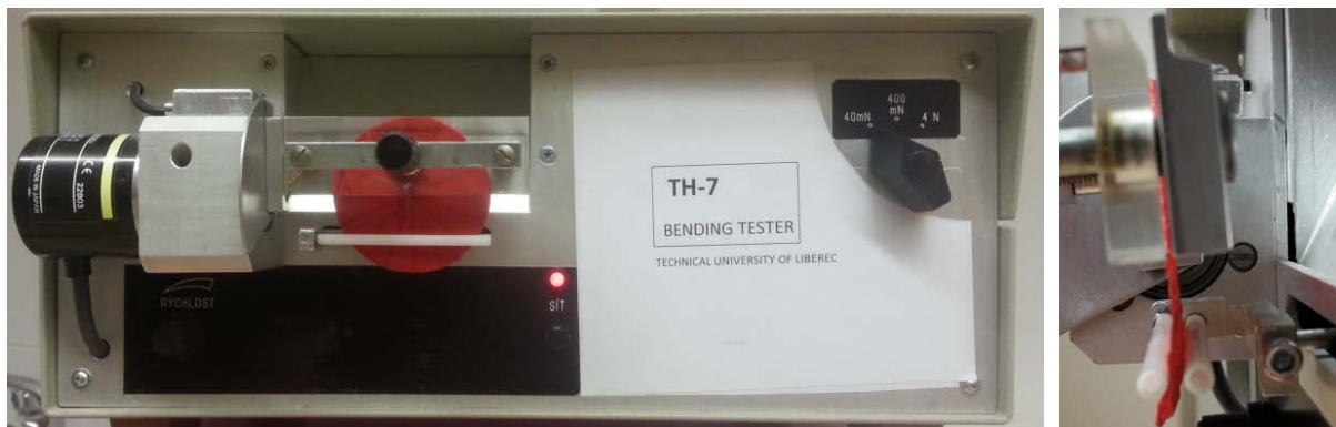
Figure 3. Specimen clamped in the TH-7 bending tester, front and side view
