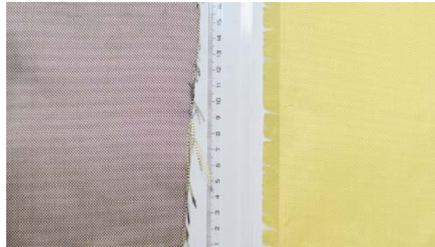
Figure 1. Kevlar with PVD surface treatment (left) and Kevlar without surface treatment (right)
