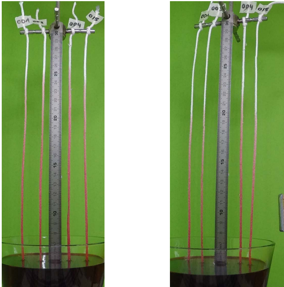
Figure 2. Results of the capillary rise height after 30 minutes in methyl ester with C 10-12 (left) and C 12-14 (right).
