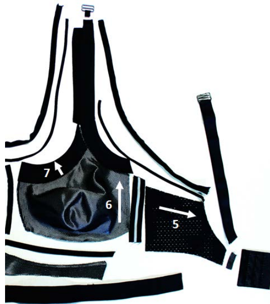
Figure 1. Unstitched Anita momentum sports bra, machine direction of samples indicated by arrow
