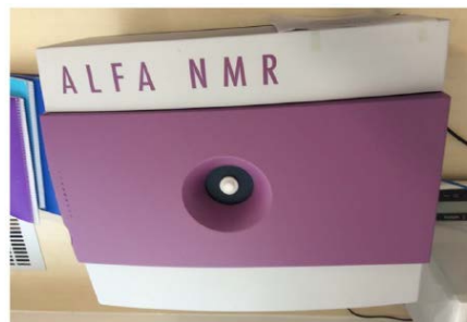
Figure 2. Lenzing-instruments Alfa NMR testing instrument for spin finish level
