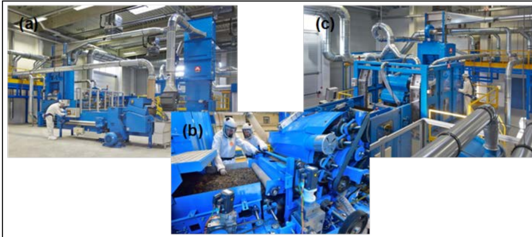
Figure 1. rCF nonwovens line, (a) tearing unit, (b) roller card supply and (c) roller card [4].
